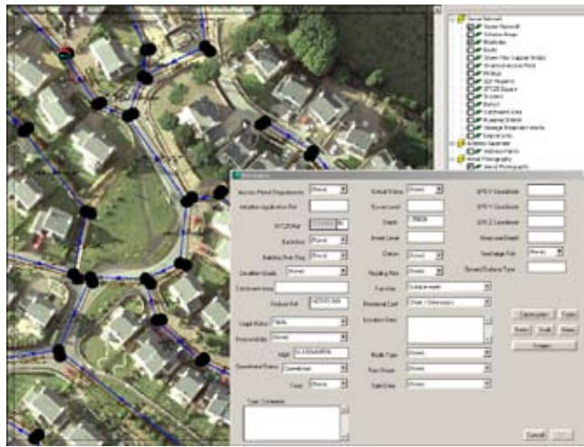
Sewer network and aerial photography in OpenWINGS
