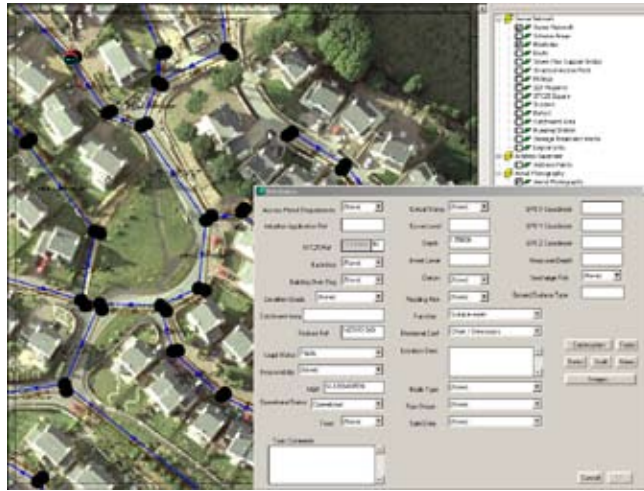
Sewer network and aerial photography in OpenWINGS
